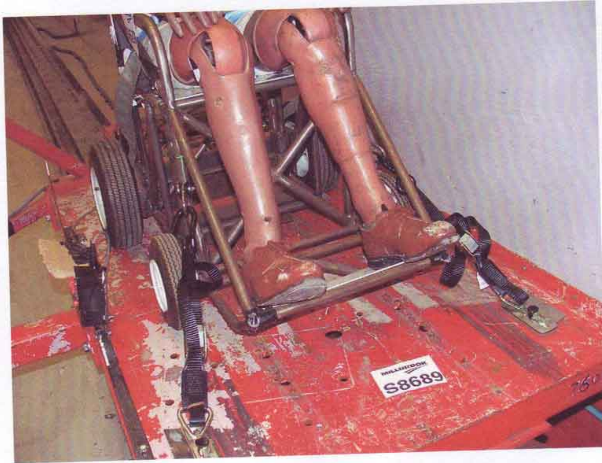
View of wheelchair front tie-downs, pre-test
