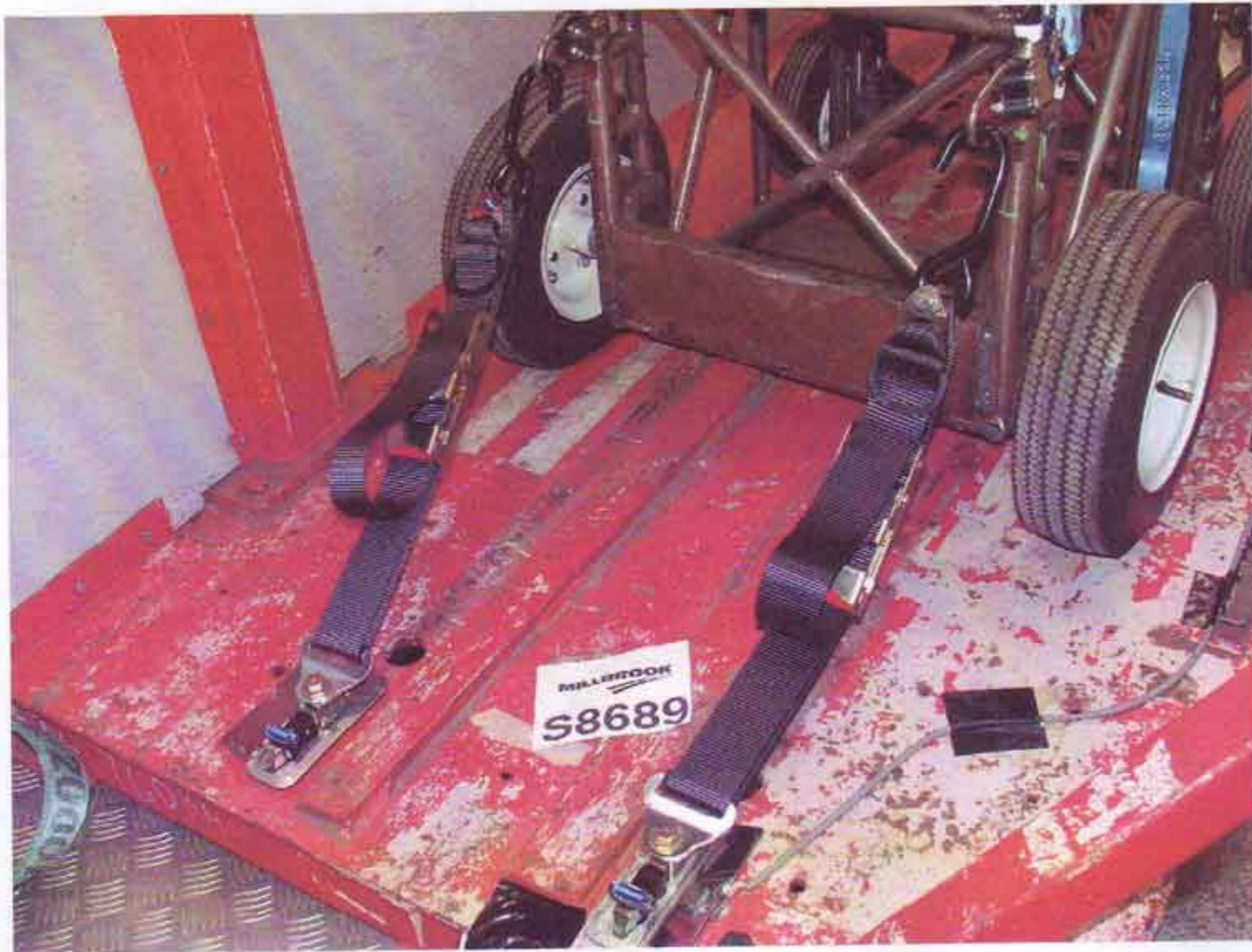
View of wheelchair rear tie-downs, post-test
