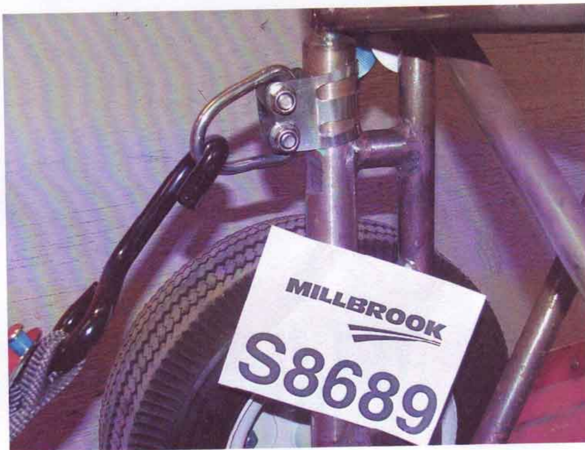
View of rear Hooki wheelchair attachment, post-test
